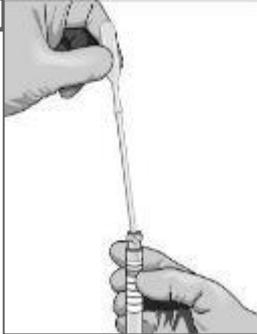
Pipette at least 1 mL of the sample using the provided pipette\*
