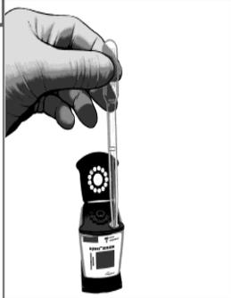
Slowly empty the pipette into the sample chamber of the cartridge
